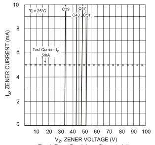
Fig. 4 Zener Breakdown Characteristics
