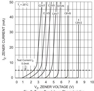
Fig. 2 Zener Breakdown Characteristics
